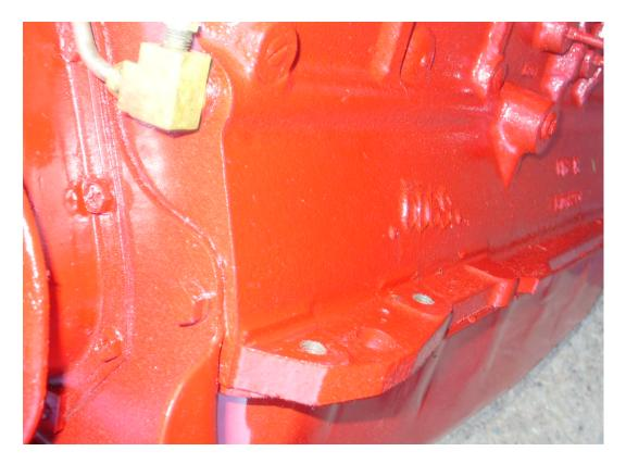
IF THE GENERATOR BOLTS ONTO THE OIL PAN RAIL WITH 2 VERTICAL BOLTS AS SHOWN IN THIS PIC, THEN IT IS A 1939-54 OR 1955 FIRST SERIES ENGINE.
